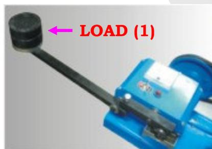
A cantilever arrangement is provided to hold and apply load on the steel billet.
